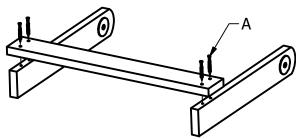
**3)** Attach Back Support Brace (shorter piece) to Back Support Sides with four A screws.
